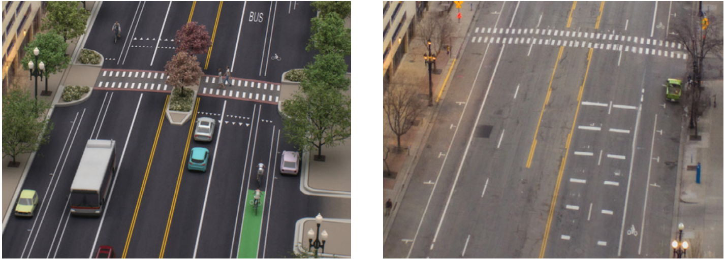
Figure 14: Mid-Block Crosswalk Example from a Redesign of 200 South in Salt Lake City
