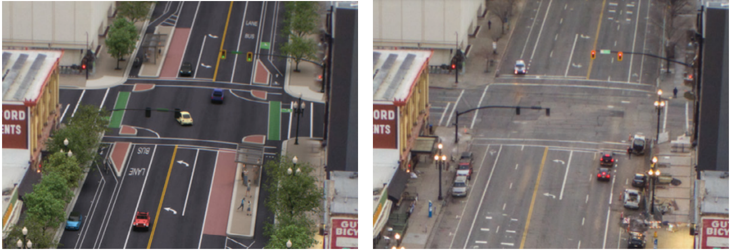
Figure 12: Example of a Complete Streets Design from 200 South in Salt Lake City
